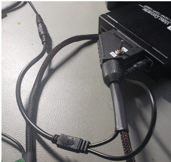
4. Install the SCART cable in to the HDMI adapter.
